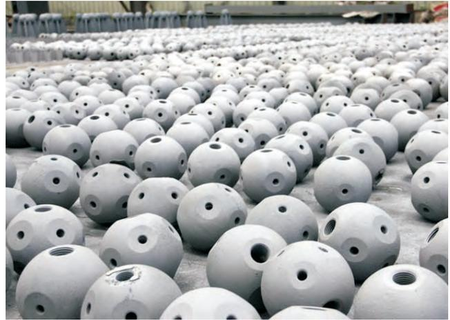
Connection ball with bolts hole for truss frame.
