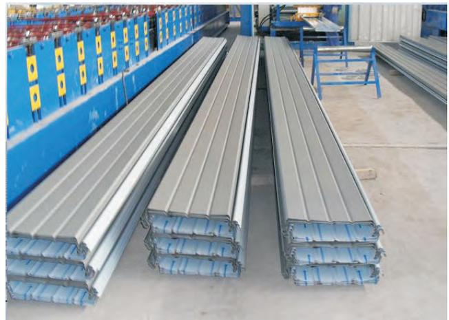
Weather resistance Al-Mg-Mn panel for structure roof.
