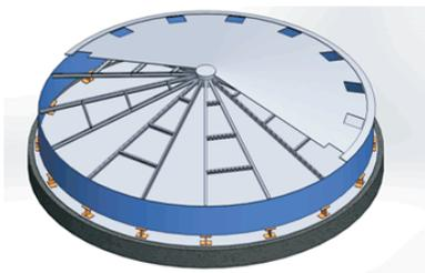
4. Install lifting device of tank, including upright column, electronic chain hoist, piston ring, lifting eye, and so on
